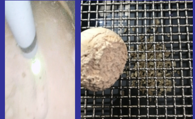
laser fiber activated to perform lithotripsy, with residual stone fragments collected under the mesh in the bench-top model
