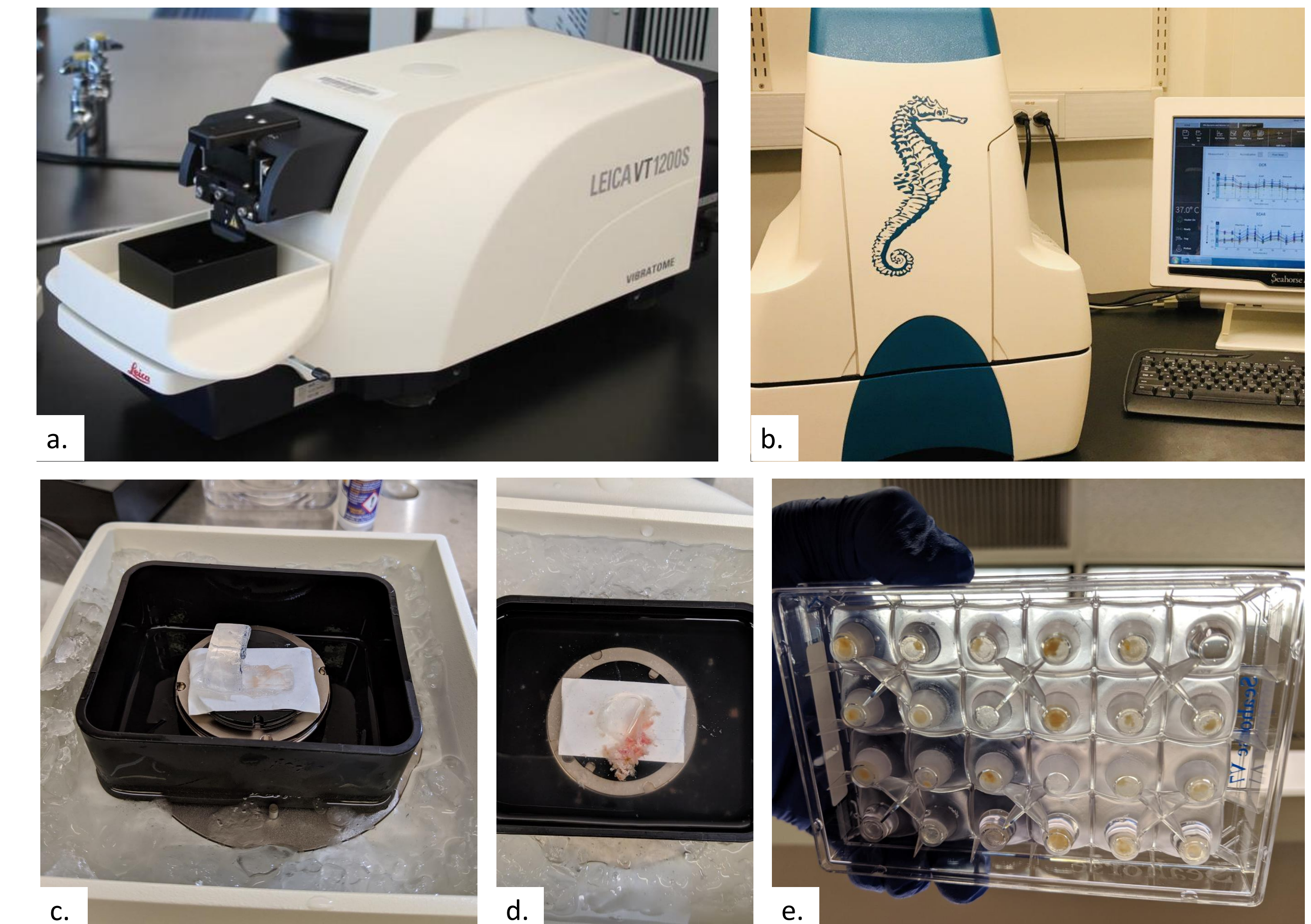
Figure 5. We developed a novel tissue slicing method for the soft PCa tumor with the (a.) Leica VT1200S microtome. (c.) Agar gel tissue "backboard" and high blade amplitude were critical in acquiring (d.) PCa tissue slices for (b.) the Seahorse XF analyzer (e.) Islet Capture Microplate samples.
